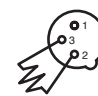
Termination reduces signal errors and avoids signal transmission problems and interference. It is always advisable to connect a DMX terminal, (Resistance 120 Ohm 1/4 W) between PIN 2 (DMX-) and PIN 3 (DMX +) of the last fixture.
